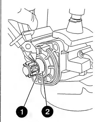
Disassembling drive-end bearing
